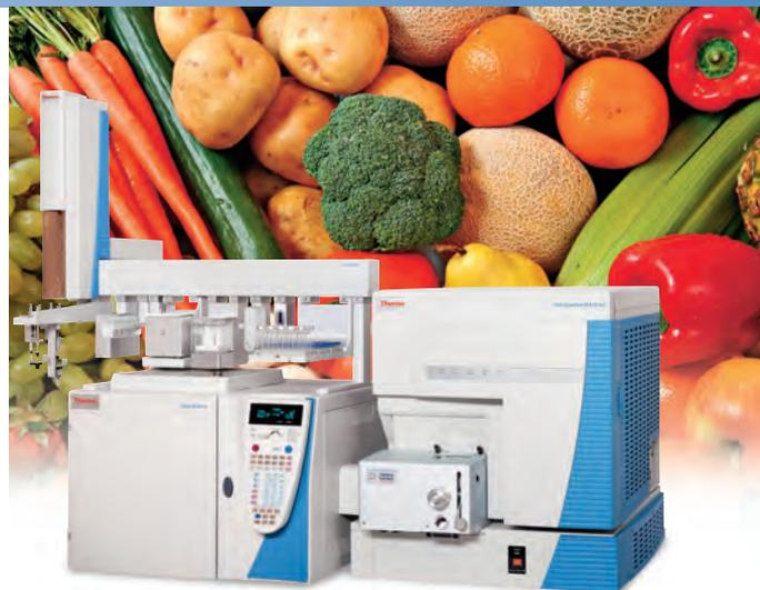
For most of the pesticide compounds included in the method, the complete list of the compounds with their respective SRM transitions have been downloaded from the Pesticides Method Reference CD (provided with the manual p/n 120390) into the instrument acquisition method. Each transition has been determined for optimal sensitivity and selectivity, with the complete list documented for TSQ Quantum XLS users.
