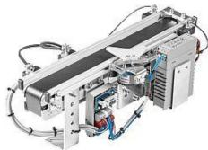
with freely positionable DC motor. It is suitable for transporting and separating workpieces with a diameter of 40 mm (e.g. "Bodies" or "Cylinder for assembly" workpiece sets). The module is supplied fully assembled.
