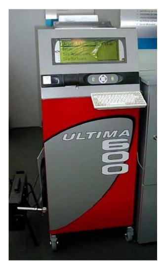
This device is new, as it can fulfill both the function of the exhaust gas analyzer, the opacity of the meter as well as a diagnostic tool. As an exhaust gas analyzer, Ultima 600 is available in version 4 gas intended for petrol engines or the kit for petrol and diesel. As a diagnostic tool, Ultima 600 will contain a reader EOBD used to read:
