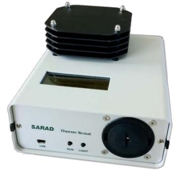
The instrument allows the simultaneous activity concentration measurement of Radon ( $Rn222$ ) and Thoron ( $Rn220$ ) based on a diffusion type measurement chamber.
