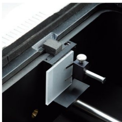
Solid sample holder to determine transmission characteristics
