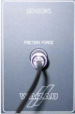
Plug in a sensor's plug carefully to prevent the pins of the multi-pole plugs from bending which may cause a bad electrical contact or no contact at all.
