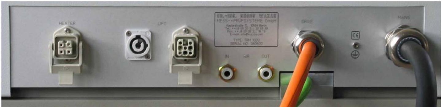
Rear side of the control rack with connections for lead, drive, lift, heater, and compressed air (IN/OUT)
