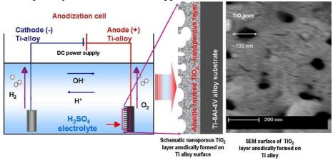
Schematic presentation of nanoporous oxide formation on titanium alloy.
